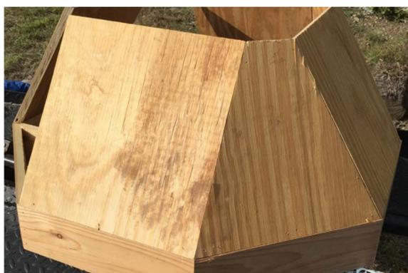
After the frame was built, the skirting then needed to be placed. Using a combination of rectangles and triangles, formed the covering for the sewing machine. These cuts were at a 36 degree cut to the angle attached to the frame and a 22.5 degree cut to attach the pieces together. Wood glue and nails were also used for support.
