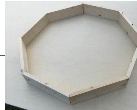
After the cuts the piece was glued and nailed for support. This part of the piece will be put under the most stress, so by giving double support the piece has a longer life span.
